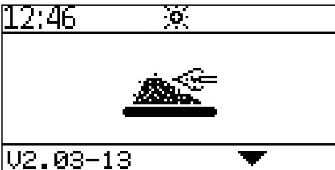
After the fire protection device has been opened, the ignition process starts and the symbol for ignition is displayed.
