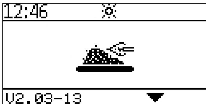
After the fire protection device has been opened, the ignition process starts and the symbol for ignition is displayed.
