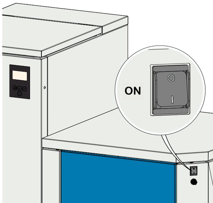
After switching on, the boiler starts (after approx. 10 seconds).
