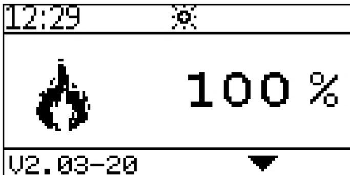
On completion of the ignition process (can last up to 15 minutes), the symbol for heating at full power appears. The boiler is now heating at full power.
