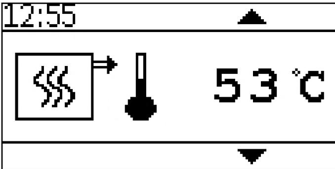
Display of the current boiler temperature
