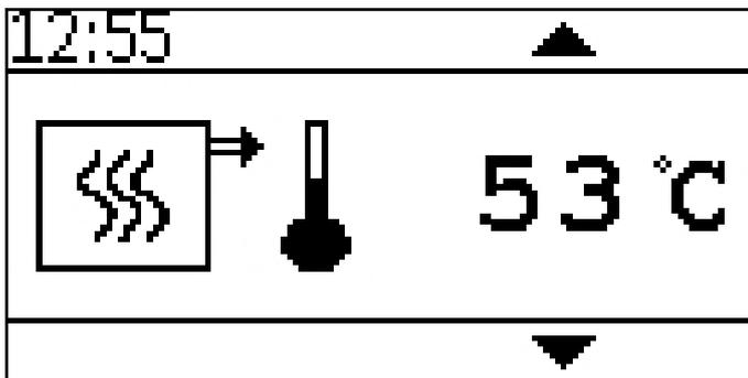
Display of the current boiler temperature
