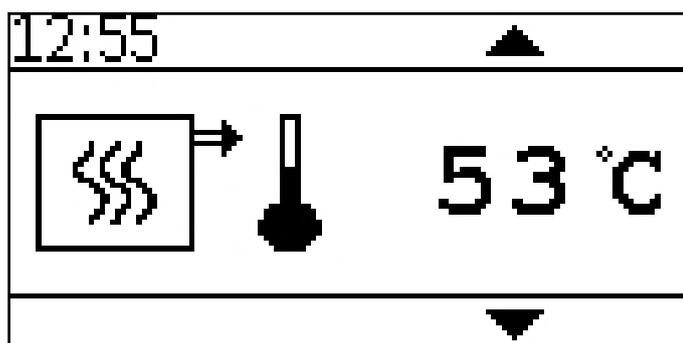
Display of the current boiler temperature
