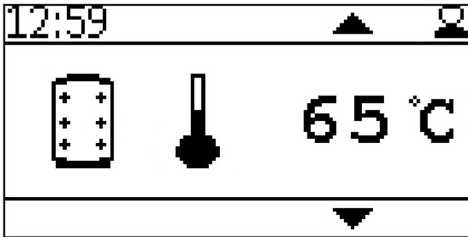
Display current accumulator temperature.
