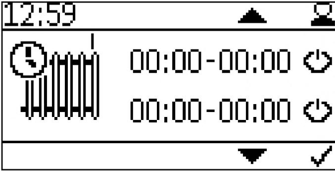
Setting the time programm of heating circuit 1.
