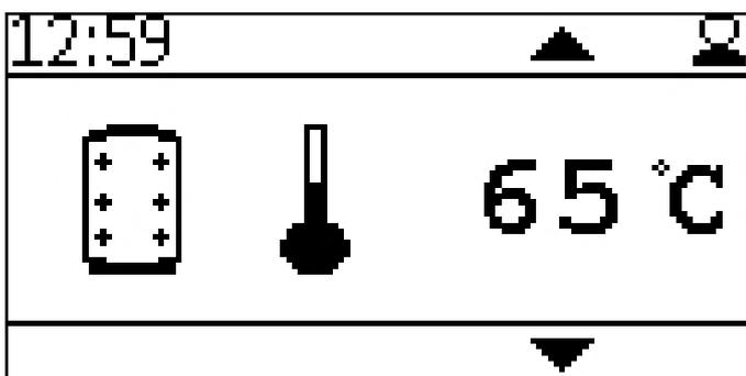
Display current accumulator temperature.
