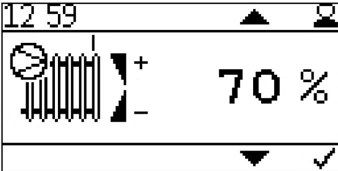
Setting the power of heating circuit pump 1.
