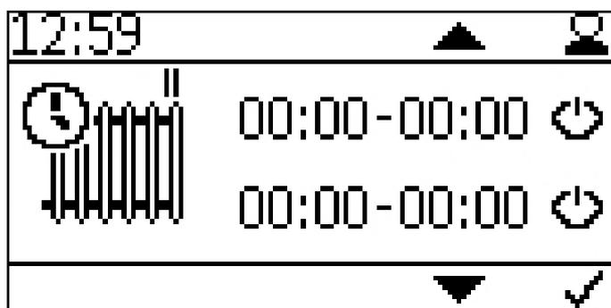
Setting the time programm of heating circuit 2.
