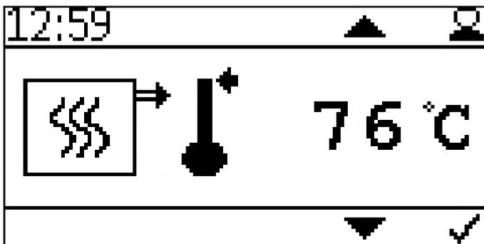
Setting of the boiler switch off temperature.
