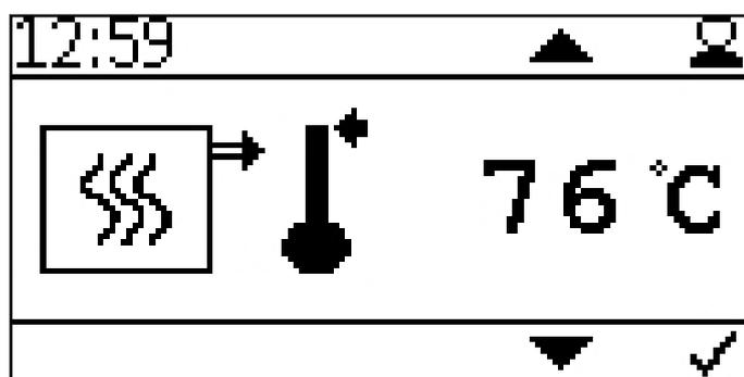
Setting of the boiler switch off temperature.
