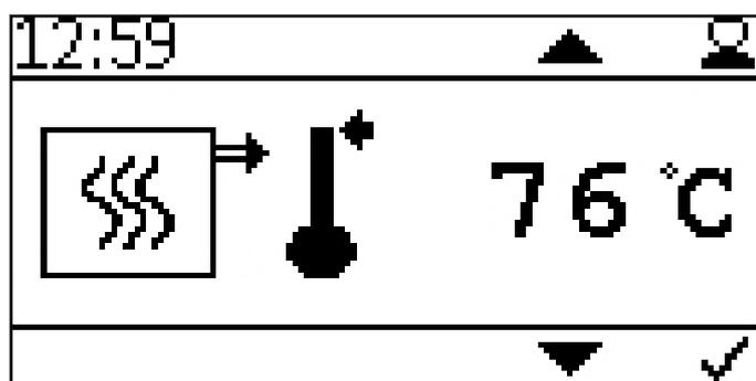
Setting of the boiler switch off temperature.
