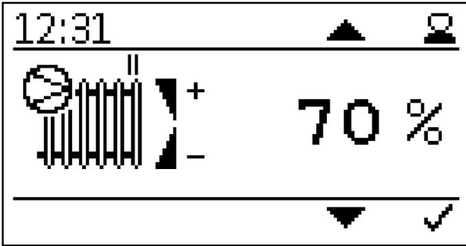
Setting the power of heating circuit pump 2.
