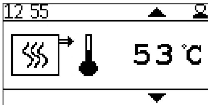
Display of the current boiler temperature
