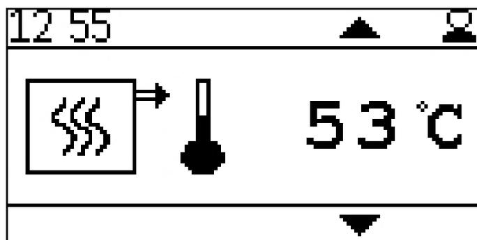
Display of the current boiler temperature
