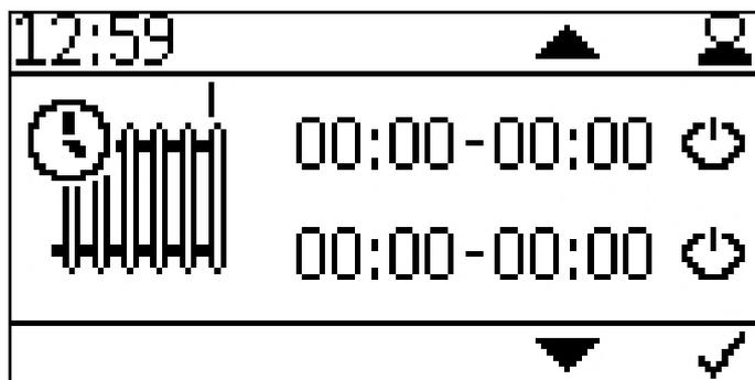
Setting the time programm of heating circuit 1.
