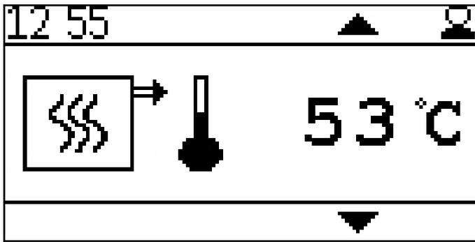
Display of the current boiler temperature
