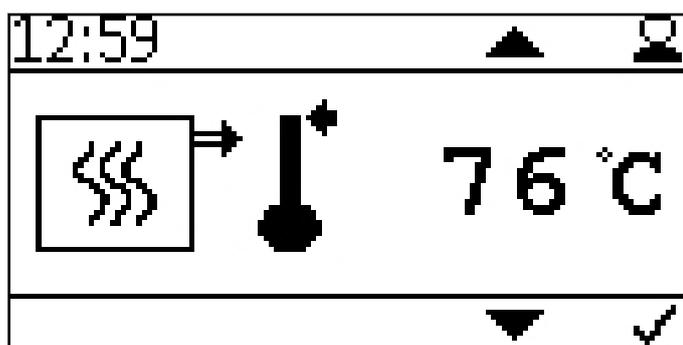
Setting of the boiler switch off temperature.
