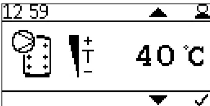
Setting pump release temperature of the heating circuit.
