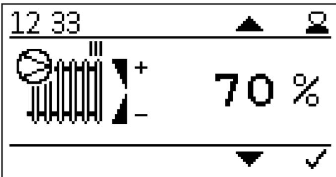
Setting the power of heating circuit pump 3.
